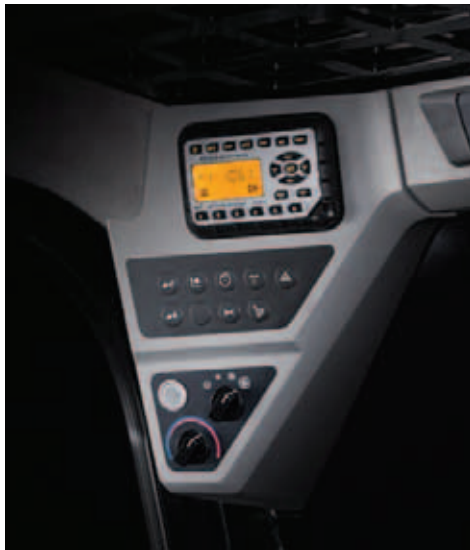
Machine option controls are ergonomically placed at roof level in the operator's line of sight.
