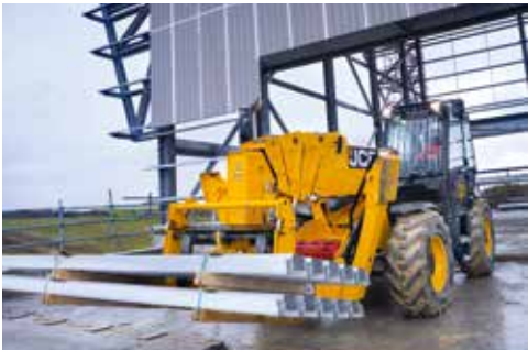
Boom mounted low in chassis gives excellent visibility.
