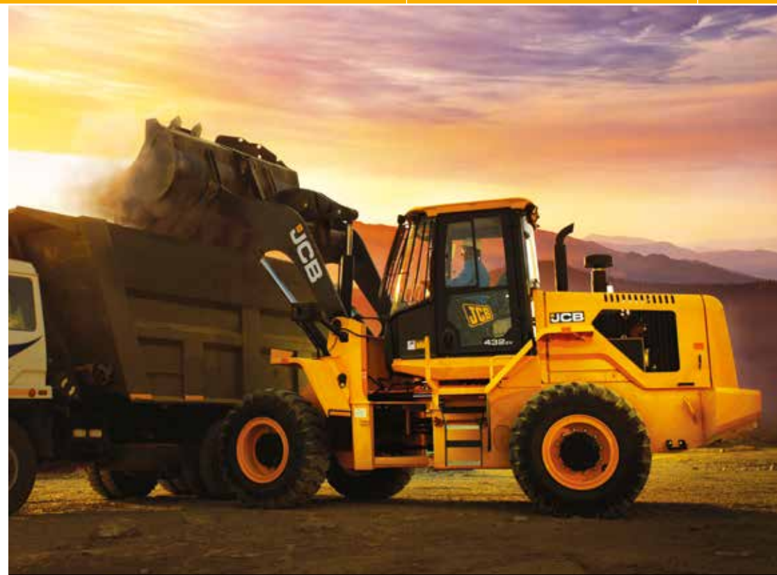
High lift loader arm.
