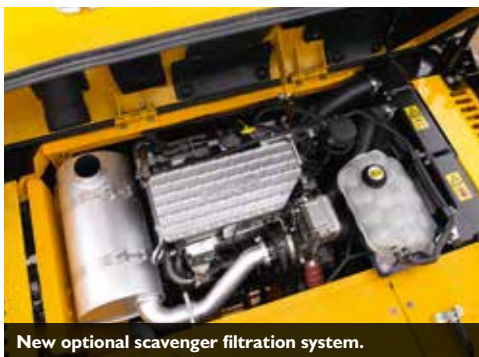
Easily accessible air filter.
