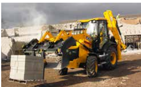
The 3CX Contractor's heavy-duty lift rams provide 3.87 tonnes of force.
