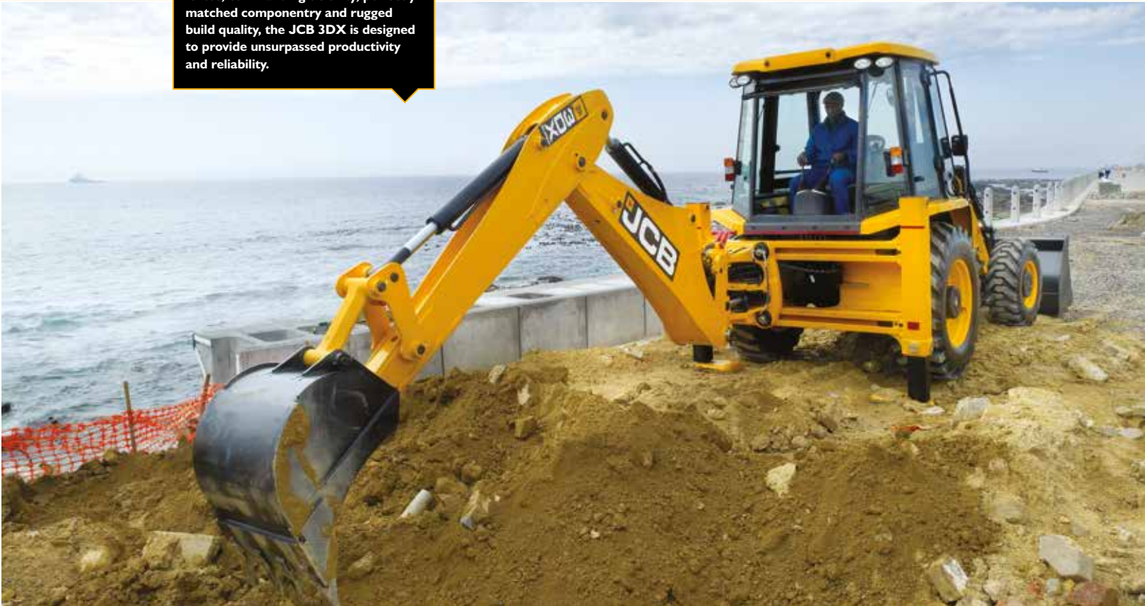
Loader arms are extremely tough, providing breakout of 6,500kgf.
