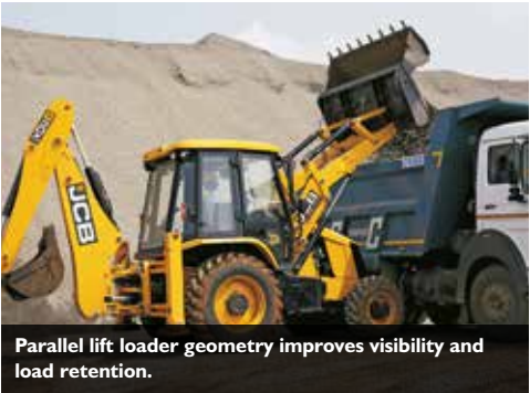
Loader arms are extremely tough, providing breakout of 6,500kgf.
