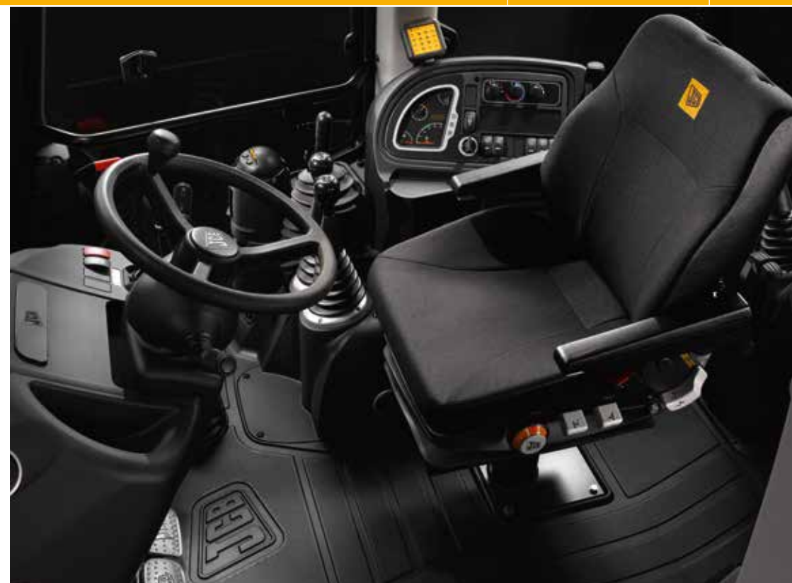
JCB's new multi-functional instrument control panel can provide current and average fuel consumption.
