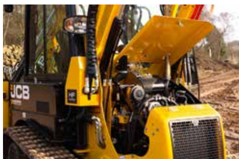
Quick, easy ground level access to daily checks.
